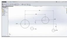
O The start point is to lay out the curves that you want to work with. Here, each gear is placed along with a tensioner floating in free space. Its position is the design goal
