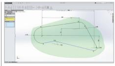
• The Path Dimension requires connected geometry. You need to trim back the circles to form a single path. Adding in construction geometry to represent the gears is also useful
