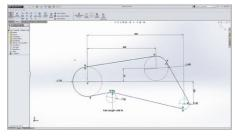
• The Path Dimension is added by selecting the path/ belt geometry from the model. Once done and okayed, the dimension is placed on the sketch and is ready for editing
