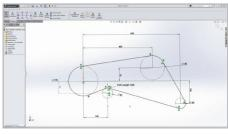
As the design progresses, dimensions and positions can be finalised, variables played with, such as ensuring enough adjustment in the tensioner
